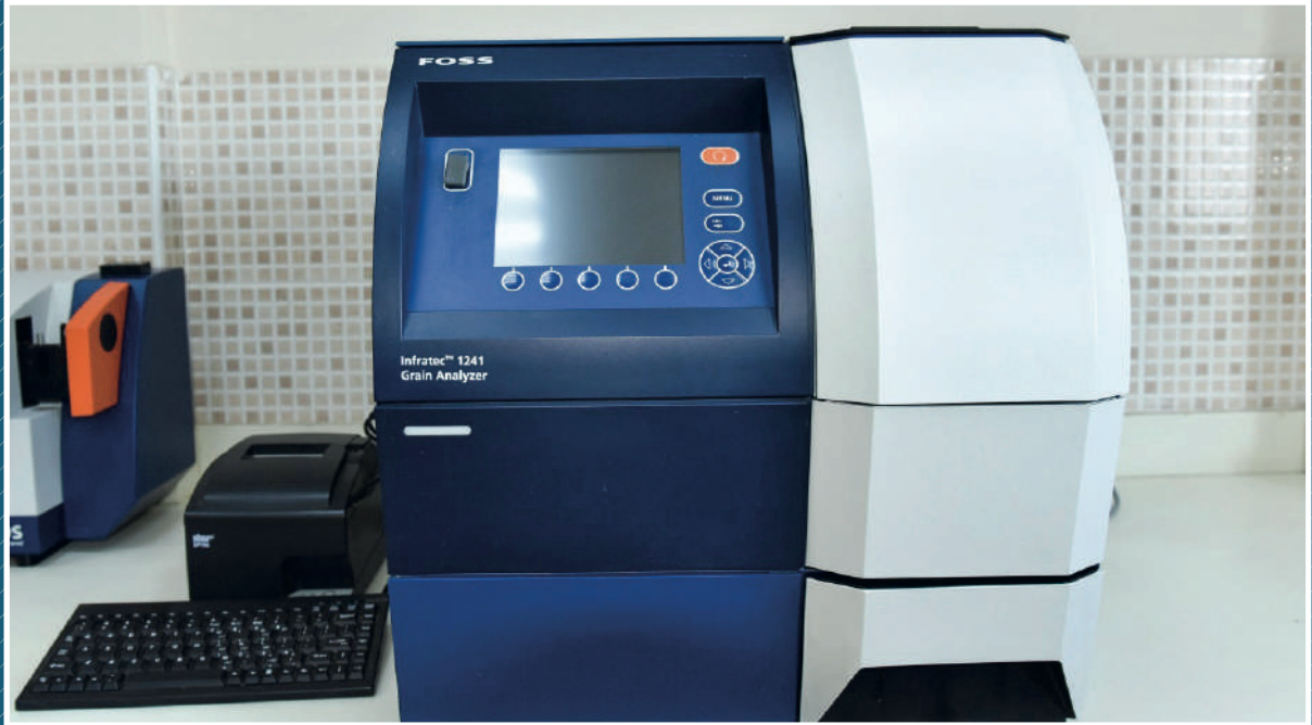
FOSS Marka INFRATEC™ 1241 Grain Analyzer Model Cihazı
